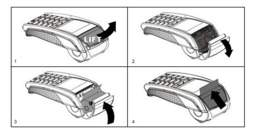
2. Unstick the end of the new roll. Leaving the end free, hold the paper roll and carefully place into the printer compartment.
